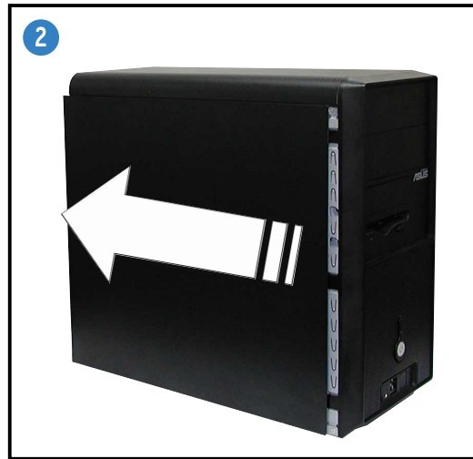
2 IMPORTANT. Repeat steps 1 and 2 to remove the other side plate.
